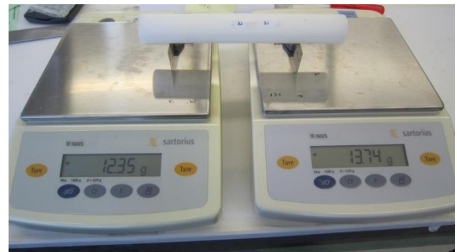
Figure 2. Measuring mass and CoG.
