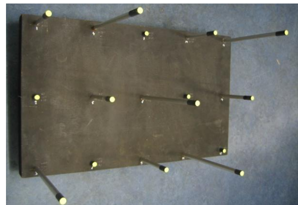
Figure 6. Calibration frame for SPR system.
