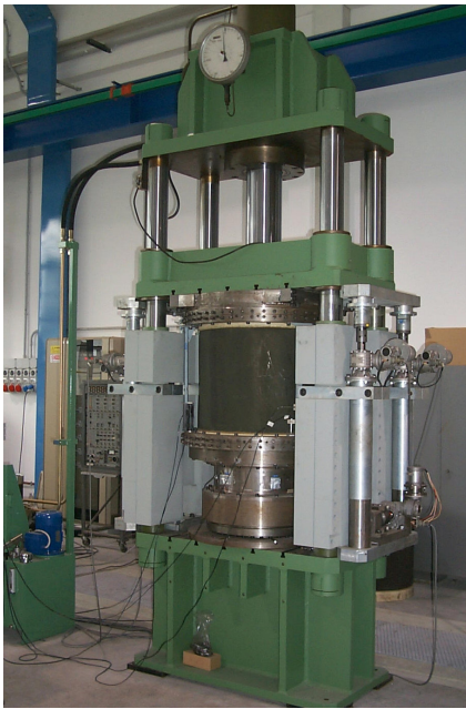
Figure 7. Buckling test facility with a cylindrical specimen inside
