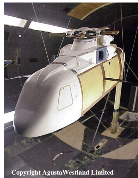
Figure 5: AW101 wind tunnel model; intake performance test at the AW Ltd wind tunnel facility.
