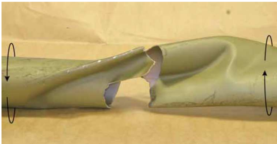
Figure 10: Torsional buckling failure example [3]
