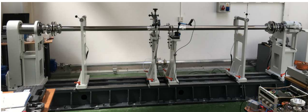
Figure 21: LDL's installation on a test bench
