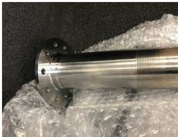
Figure 16: LDL's final shaft machined
