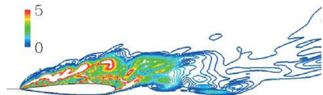
Figure 10: Example of an instantaneous flow field simulated by a hybrid RANS-LES turbulence model for \alpha = 170^\circ .
