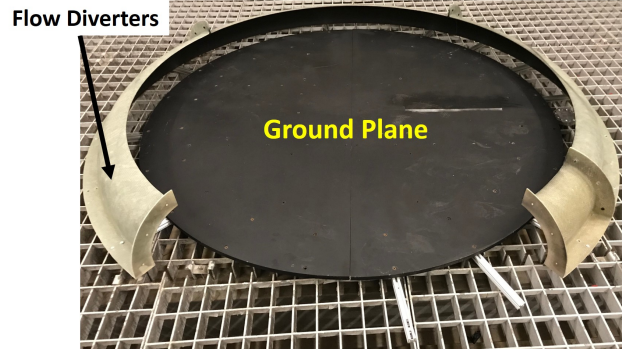
Fig. 2: Photograph of the ground plane with flow diverters [19].
