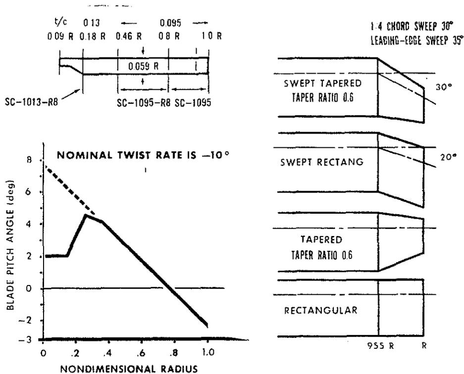
Figure 9. Blade and Tip Geometry
