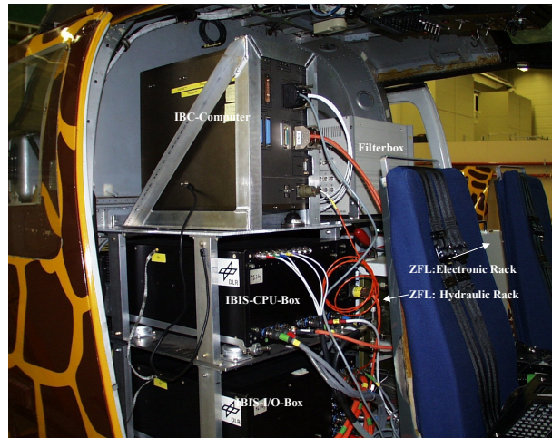
Fig. 3: Integration of IBC computers into the helicopter
