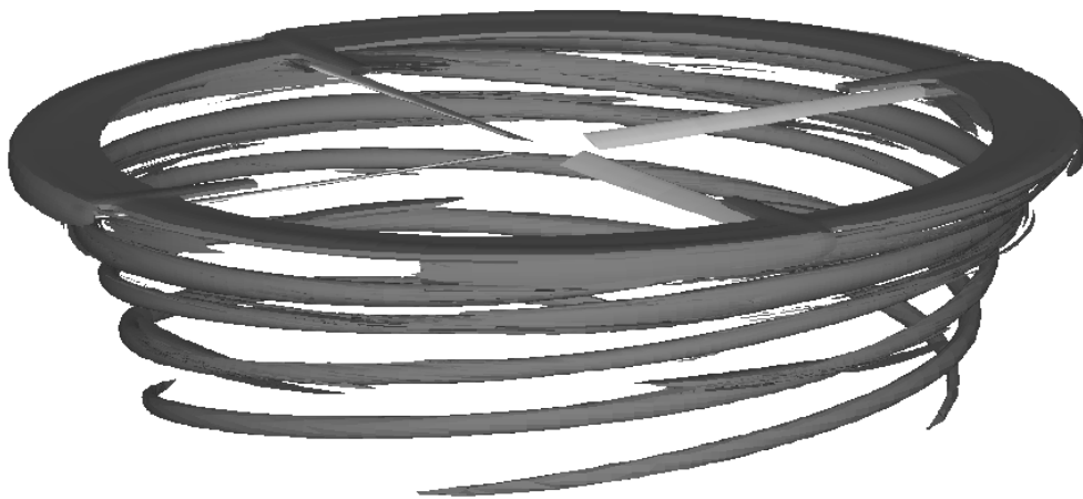
Fig.11 Iso-vorticity(0.2) surfaces of the tip (Vortex Tube Model)
