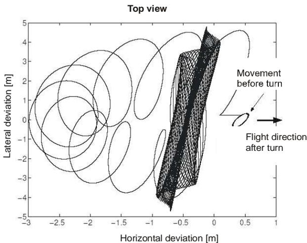
Fig 7: Modelled trajectory of the Helipod during a 180° turn in top view
