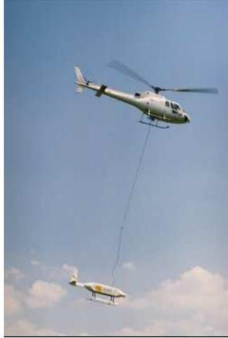
Fig 2: Helipod towed by a helicopter
