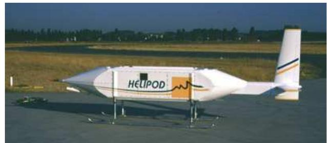
Fig 1: Helicopter-borne probe Helipod
