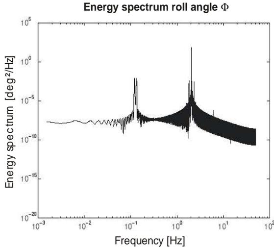
Fig 4: Energy spectrum of the roll angle  $\Phi$  after a lateral deflection
