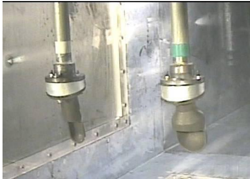
Figure 5: Ventilation outlets V0 (left) and V1 (right) mounted in the icing wind tunnel test section
