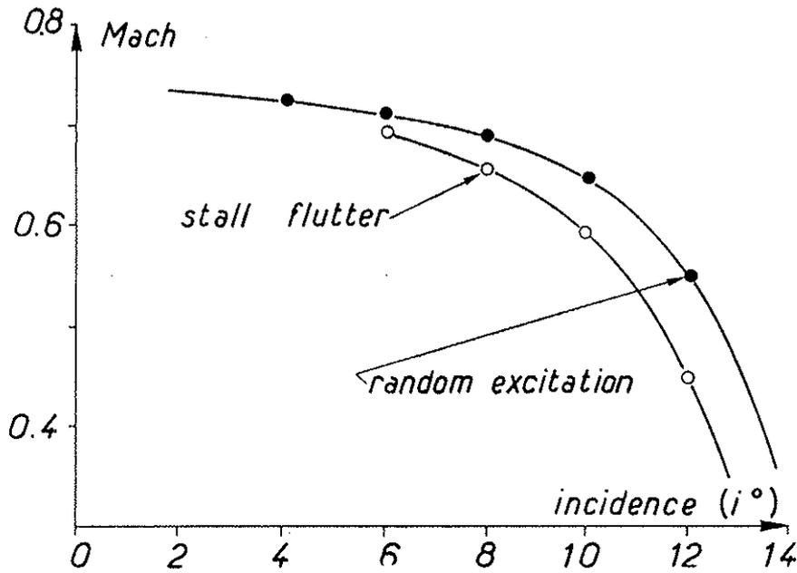
Fig. 11 - Comparison between the limiting conditions for stall flutter and for random excitation.
