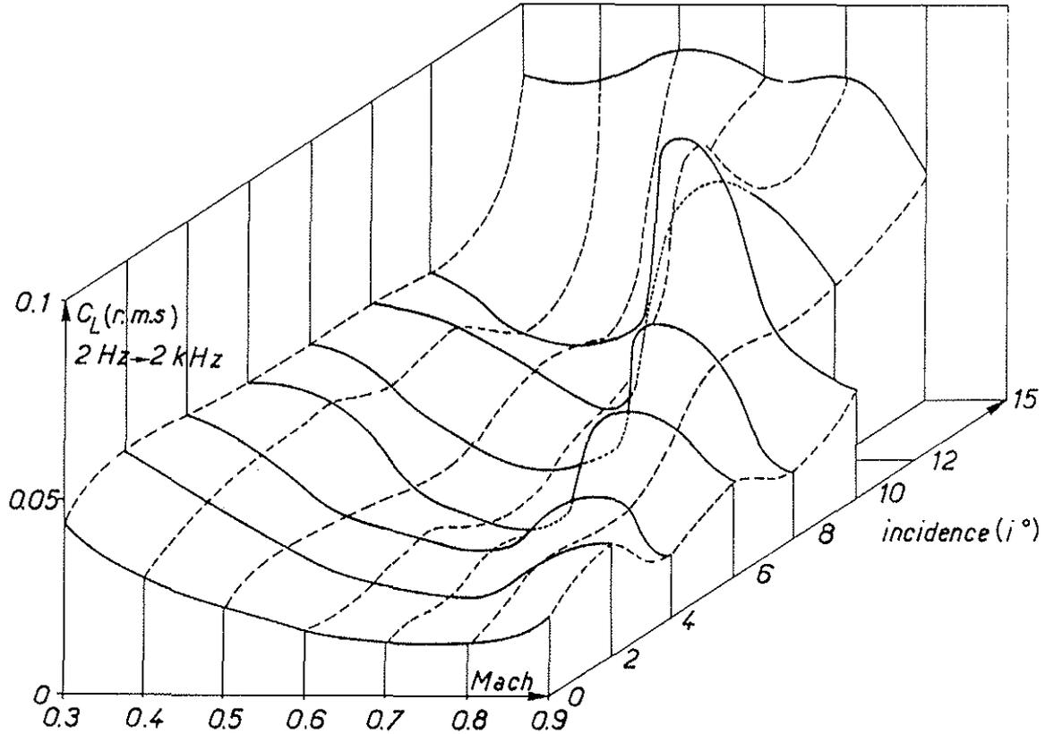
Fig. 4 - Fluctuating lift plotted against Mach number and angle of incidence.
