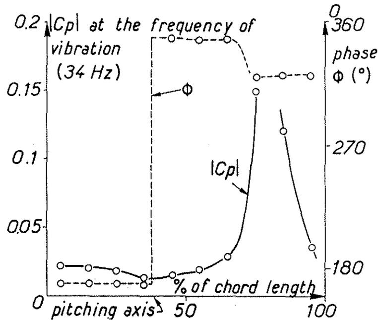
Fig. 10 - Fluctuating pressure distribution on the lower surface at  $i = 8^\circ$  and Mach 0.9.
