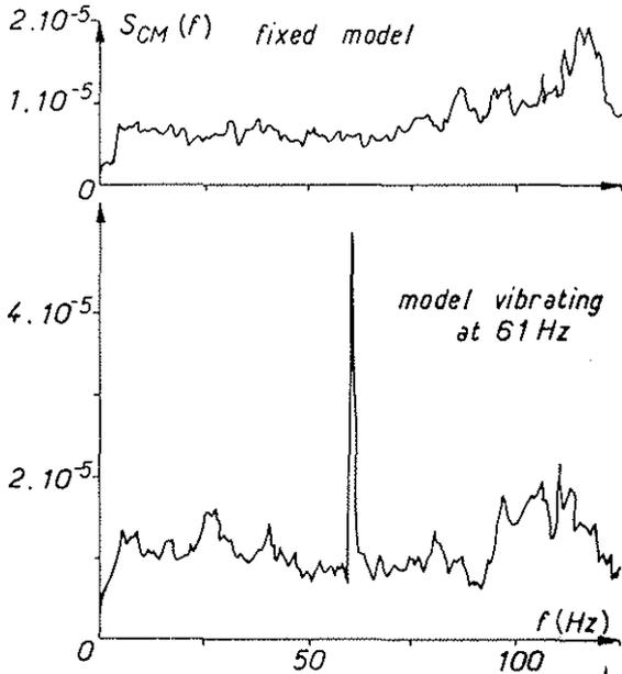
Fig. 8 - Typical moment spectra. Influence of vibrations on the separated flow pressure field.
