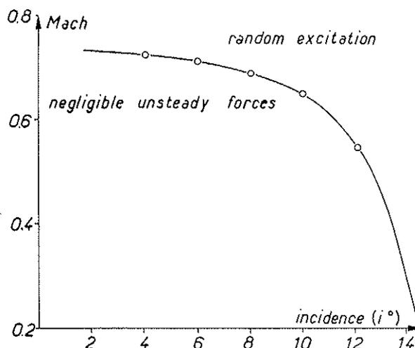
Fig. 7 - Limits of large random pressure fluctuations.
