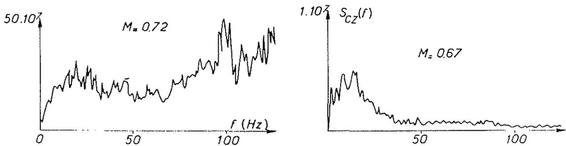
Fig. 5 - Frequency spectra at speeds below and above the separation speed -  $i = 8^\circ$ .
