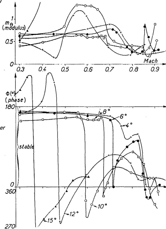
Fig. 9 -  $m_\theta$  and  $\phi$  a function of Mach number at various angles of incidence.
