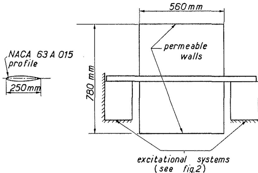
Fig. 1 - Wind tunnel and model.
