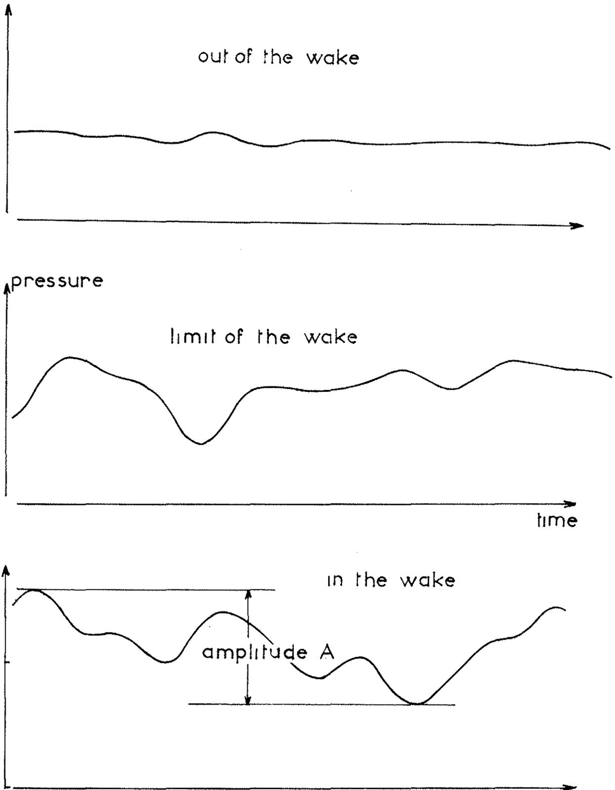
Fig 7 wake analysis by measure of pressure
