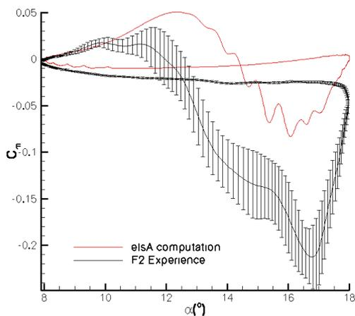
Comparison between computation with transition and experimental pitching moment coefficient for a deep stall case,  $Re=1.8M$
