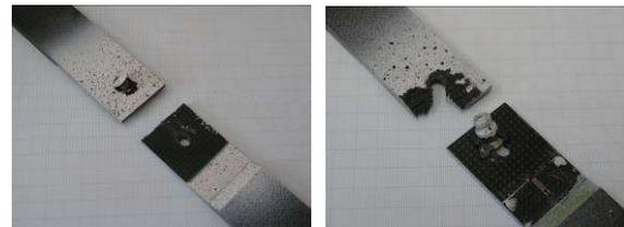
Rivet failure (0.1 m/s)    Shear out (10 m/s)
