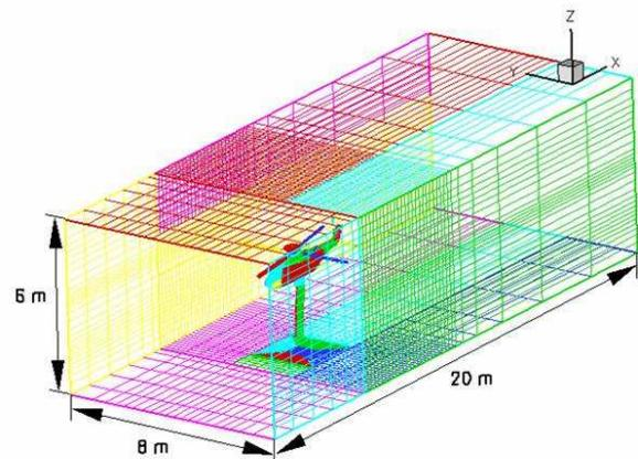
Figure 7 : GOAHEAD CFD grid system including wind tunnel walls
