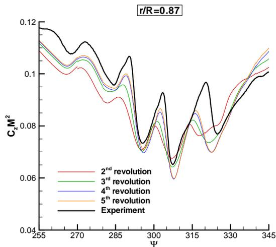
Convergence of the sectional load  $C_z M^2$  for the fine background grid
