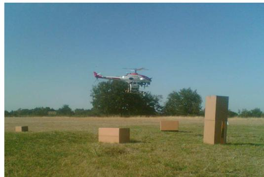
Figure 28 RESSAC autonomous landing with obstacles
