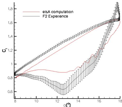
Comparison between computation with transition and experimental lift coefficient for a deep stall case,  $Re=1.8M$
