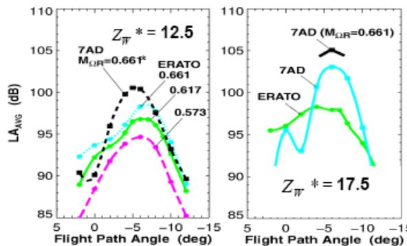
Figure 10 : 7AD-ERATO acoustic comparison at 125 km/h, DNW measurements, dBA levels: left Z<sub>b</sub> =12.5, right Z<sub>b</sub> = 17.5
