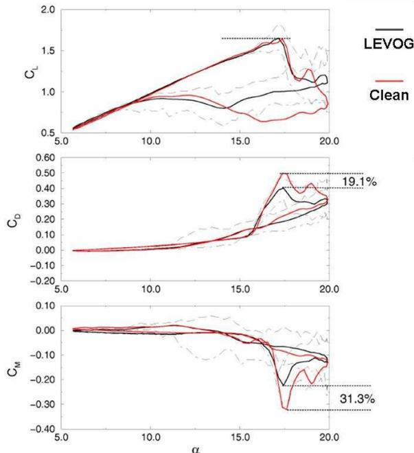
Figure 3 Measured mid-span lift-, pitching-moment- and pressure-drag hysteresis loops integrated from measured unsteady pressure distributions for a deep dynamic-stall case with and without LEVoGs ( $M=0.31$ ,  $Re=1.15e6$ ,  $\alpha=12.9^\circ+7.1^\circ \sin(\omega t)$ , red. freq. =0.1)
