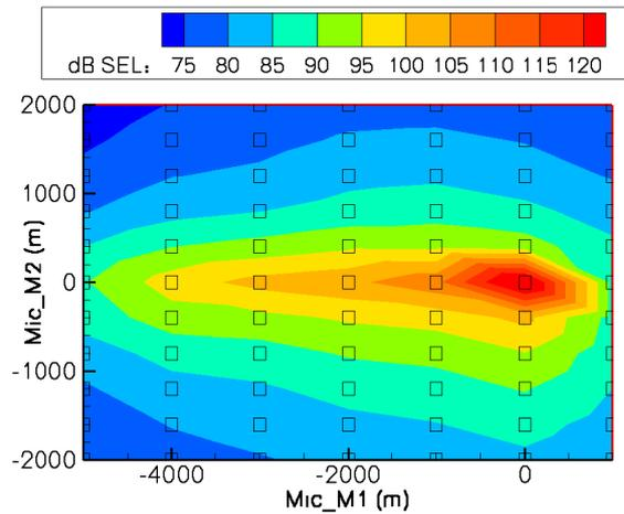
Figure 12 Ground noise footprint (SEL level) for an optimized descent flight
