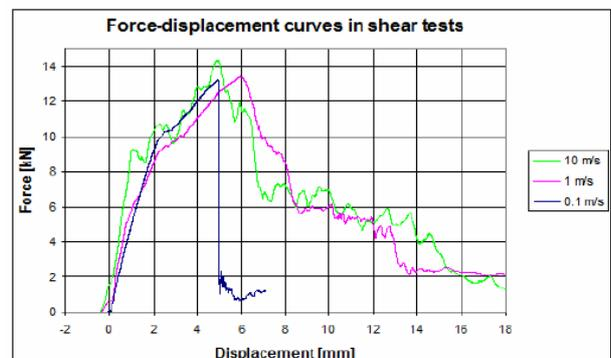
Figure 19 Dynamic shear tests on riveted composite joints showing influence of loading rate
