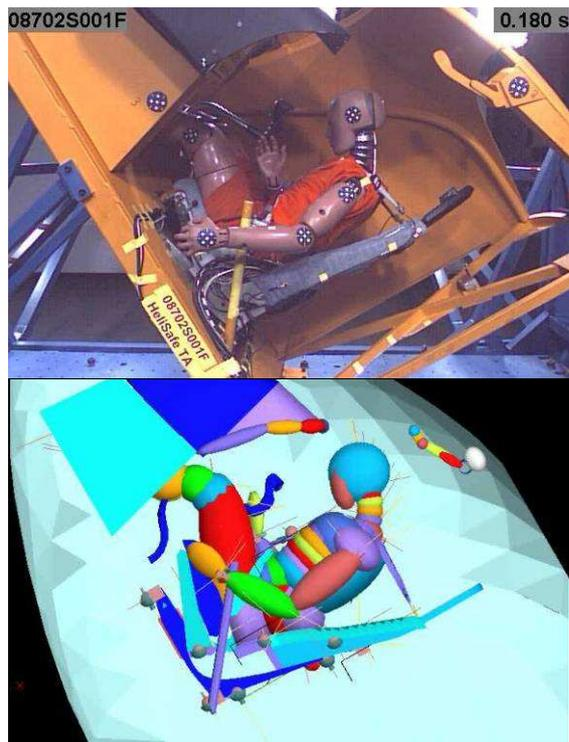
Figure 20 : Validation of cockpit model with sled test pulse representing crash load  $V_x = 12.8$  m/s,  $V_z = 7.9$  m/s, with 50% dummy and 4-Point belt
