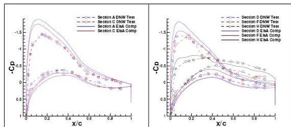
Figure 27 Experimental and numerical pressure coefficient on the inner wing (left) and on the outer wing (right) (conversion case) [26]
