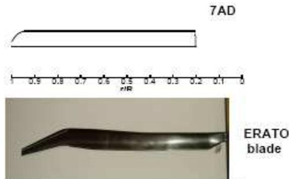
Figure 9 : ERATO shape compared to reference rotor
