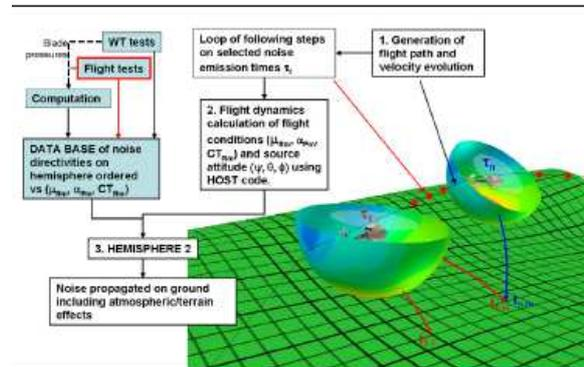
Figure 11 Schematic representation of the computational chain.
