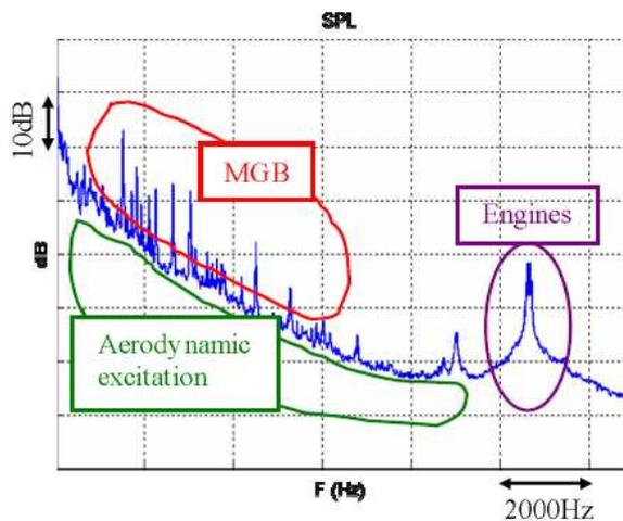
Figure 21 Level and origin of induced vibration and noise, inside the fuselage
