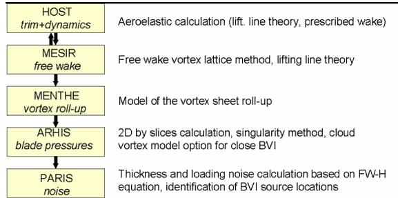
Figure 8 : HMMAP calculation chain for BVI noise
