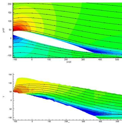
Figure 5 :Comparison of axial velocity component at  $\alpha=14.5^\circ$
