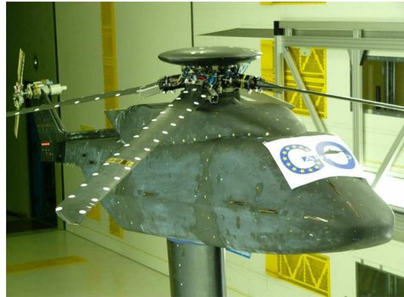
Figure 6 : GOAHEAD model in DNW wind tunnel
