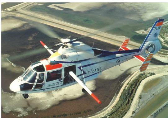
Figure 15 D6075 (DGA/CEV) with beam for measurement probes
