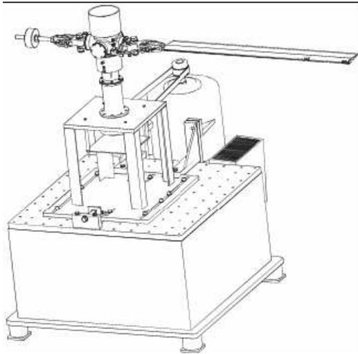
Figure 23 Centrifugal test rig
