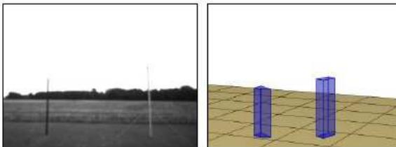
Figure 30 Example of a created map. Original left camera image (left) and resulting 3-D map of the two obstacle posts (right)
