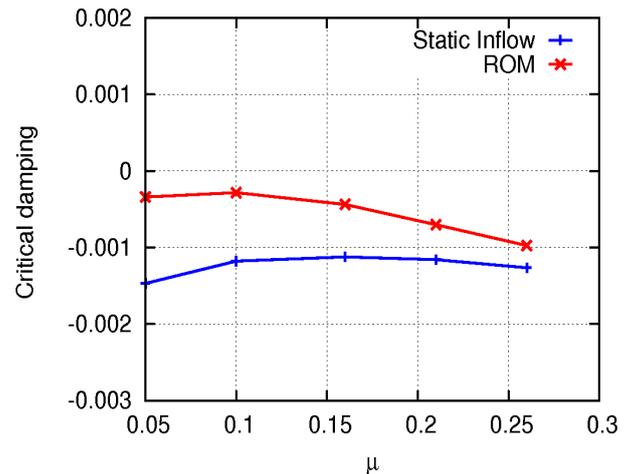
Figure 6. Critical dampings vs advance ratio.
