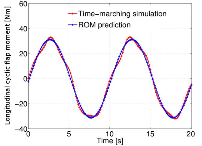
Figure 5. Comparison between time-marching BEM simulation and ROM prediction.
