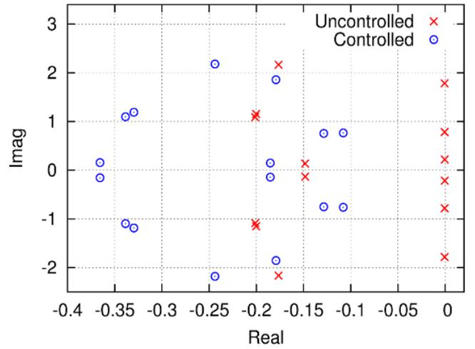
Figure 12. Controlled aeroelastic eigenvalues.
