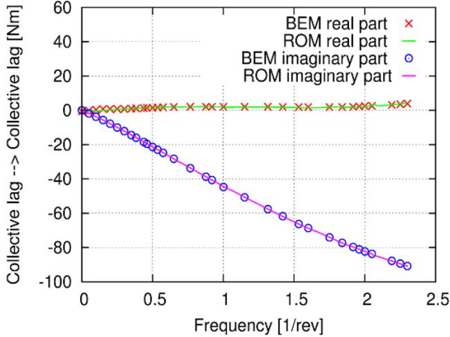
Figure 3. Transfer function between collective lag bending moment and collective lag deflection.
