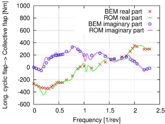
Figure 4. Transfer function between collective flap bending moment and long. cyclic flap deflection.
