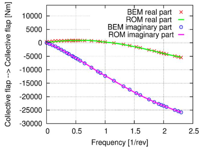
**Figure 1. Transfer function between collective flap bending moment and collective flap deflection.**
