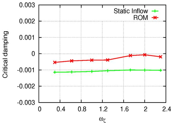
**Figure 8. Critical dampings vs lag stiffness.**
