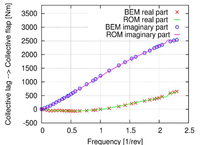
**Figure 2. Transfer function between collective flap bending moment and collective lag deflection.**
