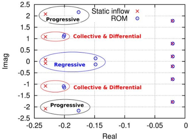
**Figure 7. Aeroelastic eigenvalues.**  $\mu = 0.16$ , 1% structural damping.
