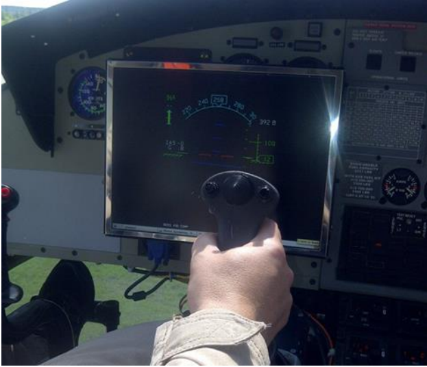
Figure 16: NRC Bell 412 ASRA – Side-Stick Testing
