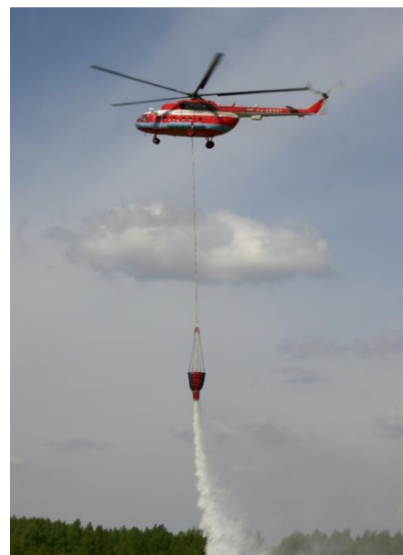
Figure1: BB-5 on a helicopter external cargo sling
