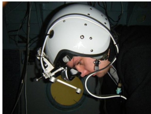
Figure 7: Cargo sling operator's visual system
