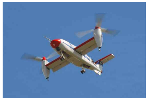
Fig. 4 Full- scale SUAV in hover mode flight
