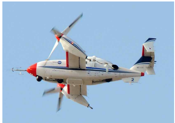
Fig. 6 Full- scale SUAV in conversion mode flight
