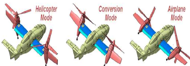
Fig. 13 Tilting concept of the extended-wing tiltrotor UAV
