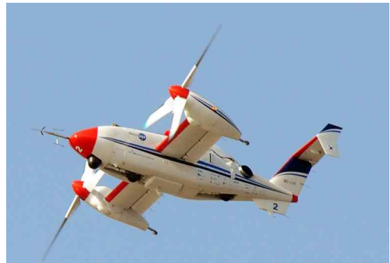
Fig. 9 Full- scale Smart UAV in airplane mode flight
