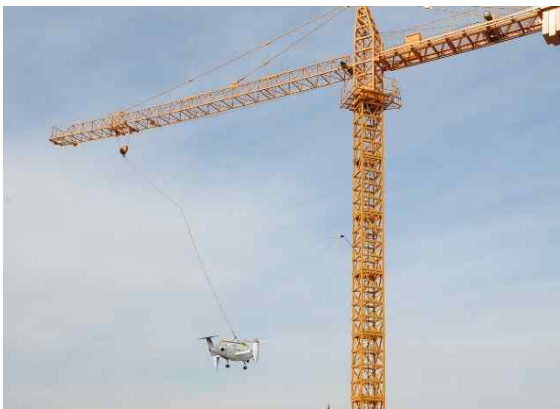
Fig. 1 Tethered flight of the full-scale Smart UAV
