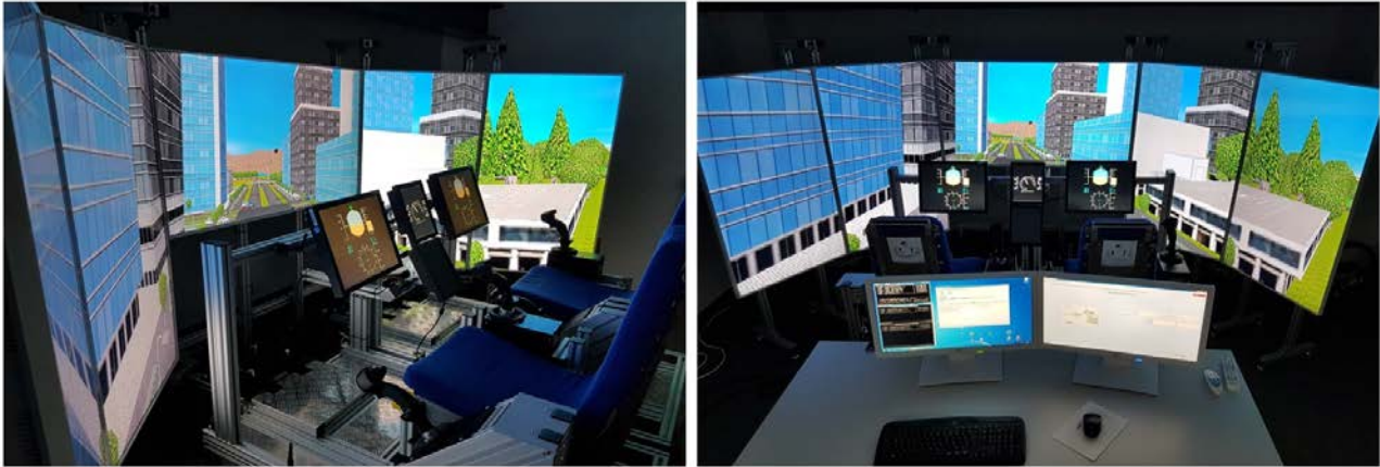
Fig. 3 - Dual Pilot Active Sidestick Demonstrator -2PASD
