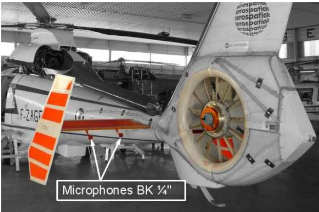
Figure 1: Microphone locations on the Dauphin 6075 for acoustic measurements
