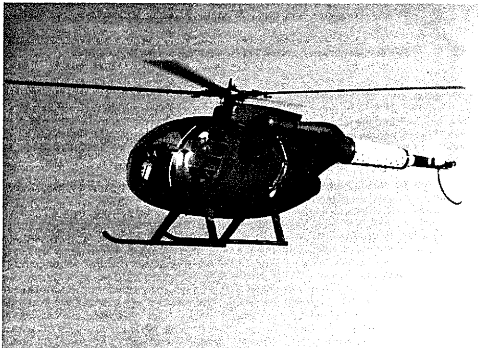
Fig. 7. Flight Test of a Circulation Control Tail Boom Installed on OH-6A.
