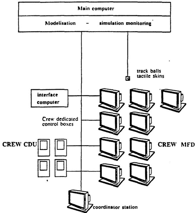
Figure 2 **HARDWARE ARCHITECTURE**
