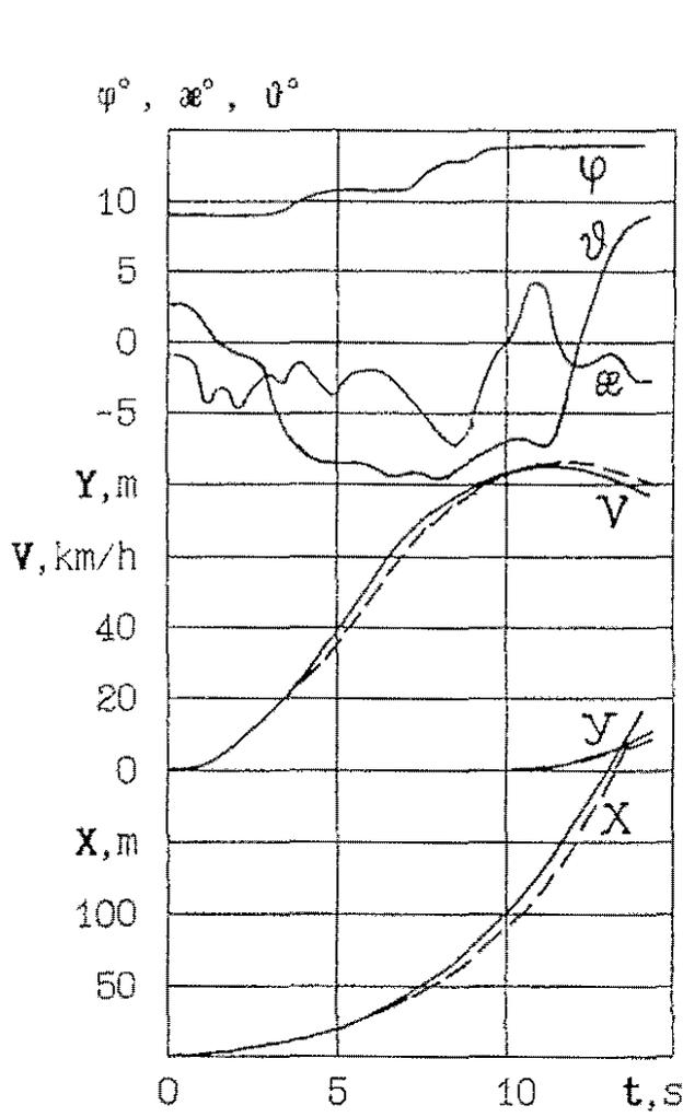
Fig.5. The main parameters of an overloaded helicopter running takeoff on the nose landing gear
