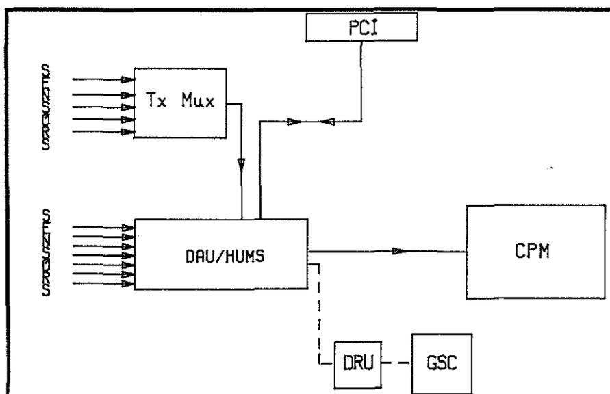
**Fig.12 Fully Integrated FDR/HUM System**
