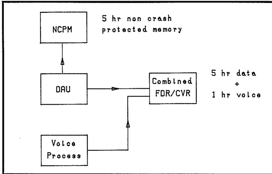
**Fig.9 Combined Voice and Data Recorder System**
