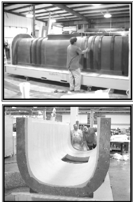
Fig. 16 Main VaRTM mold during fabrication (top) and after cure and machining of the inner surface (bottom)
