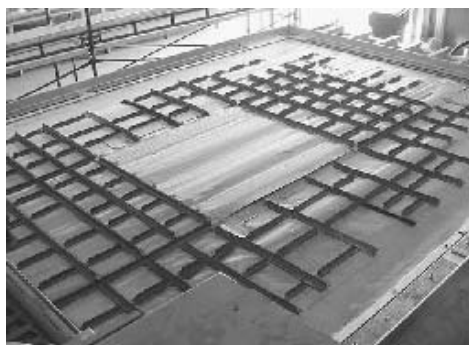
Fig. 12 Completed skin-stringer preform
