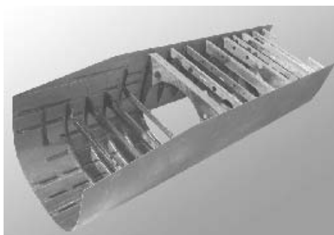
Fig. 18 The VaRTM-infused unitized sub-assembly
