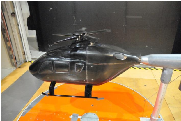
Figure 1: Helicopter model mounted in the wind tunnel test section
