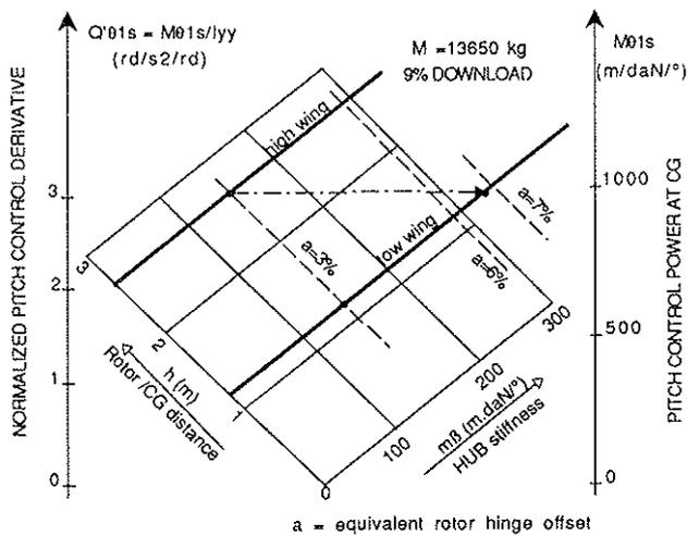
Figure 9 : Impact of wing position on pitch controllability
