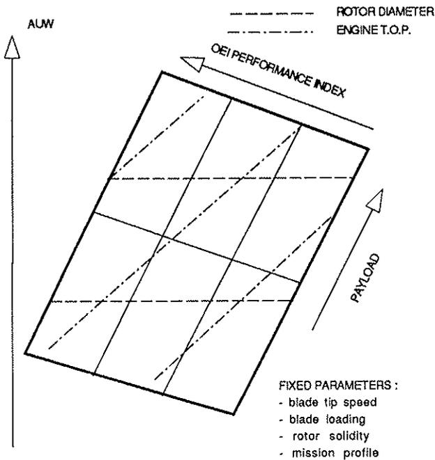
Figure 1.a : Typical helicopter sizing diagram
