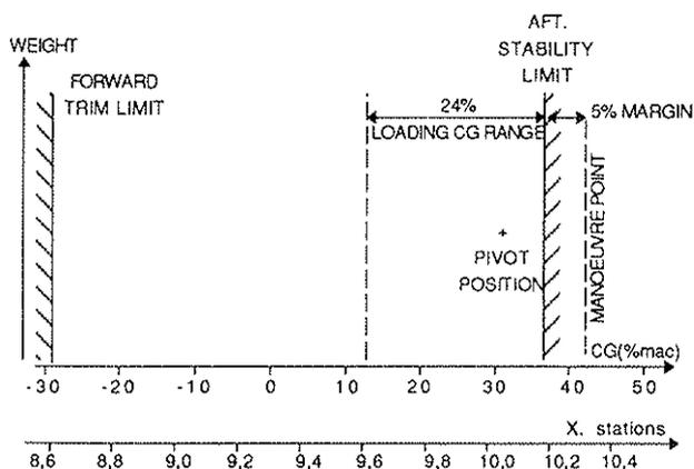
Figure 17 : Handling qualities limits in aircraft mode
