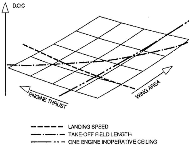
Figure 1.b : Typical airplane sizing diagram
