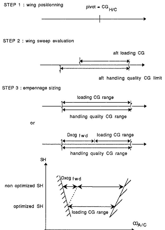
Figure 13 : Configuration optimization process
