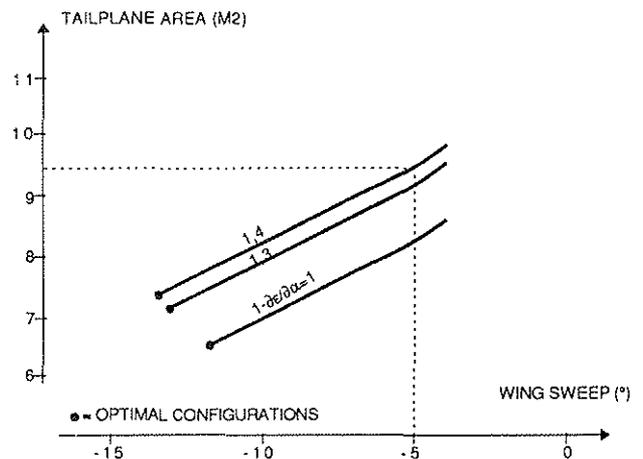
Figure 15 : Influence of sweep angle on empennage sizing
