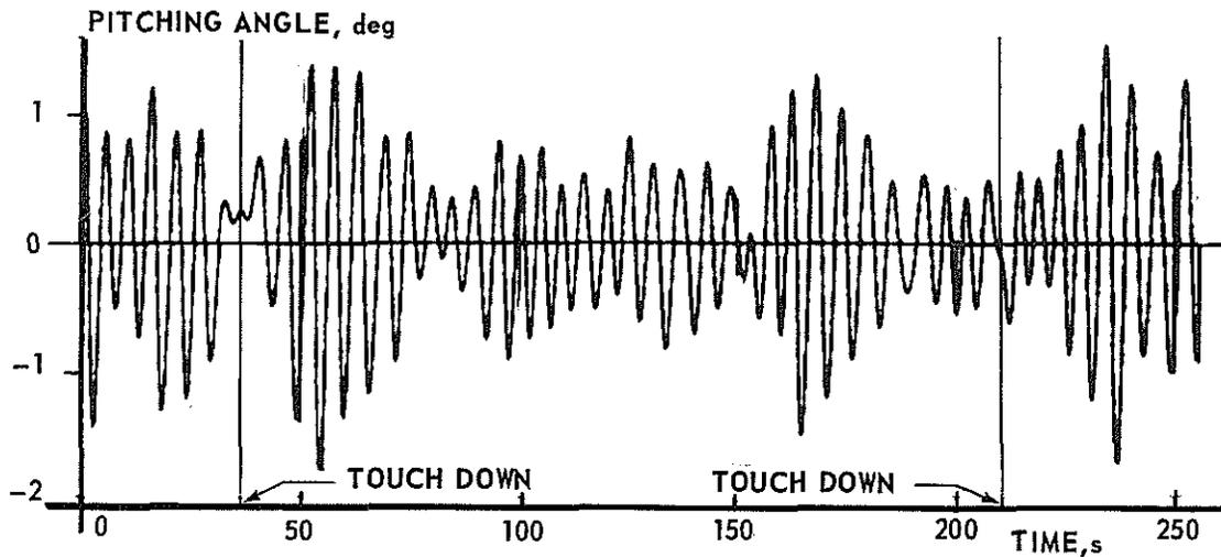
Fig. 8 Measured pitching angle of ship vs time with moment of touch down
