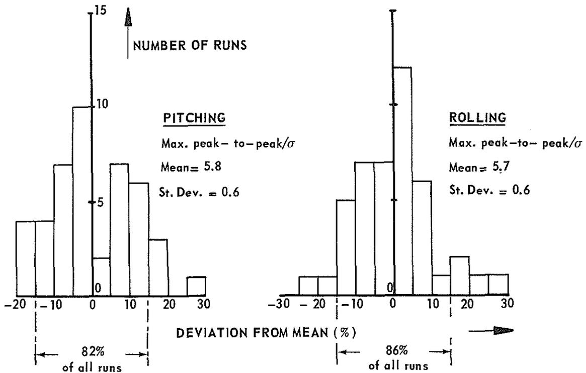
Fig. 9 Histogram of the ratio between max. peak-to-peak and  $\sigma$ -value of measured pitching and rolling angles of a ship
