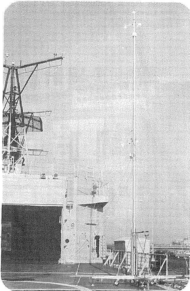
Fig. 4 Movable mast for full-scale air flow measurements above the flight deck
