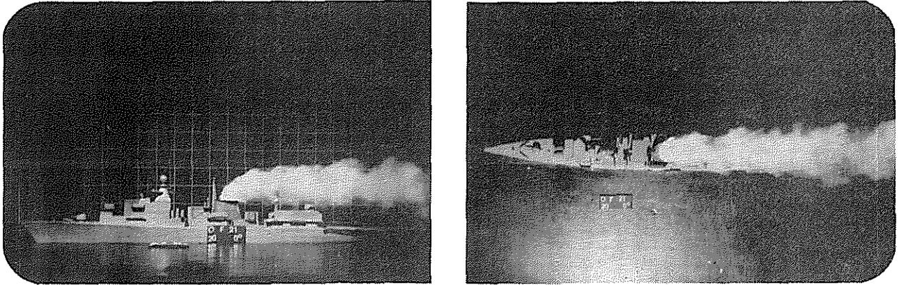
Fig. 3 Exhaust plume investigation at simulated full-power condition in a wind tunnel
