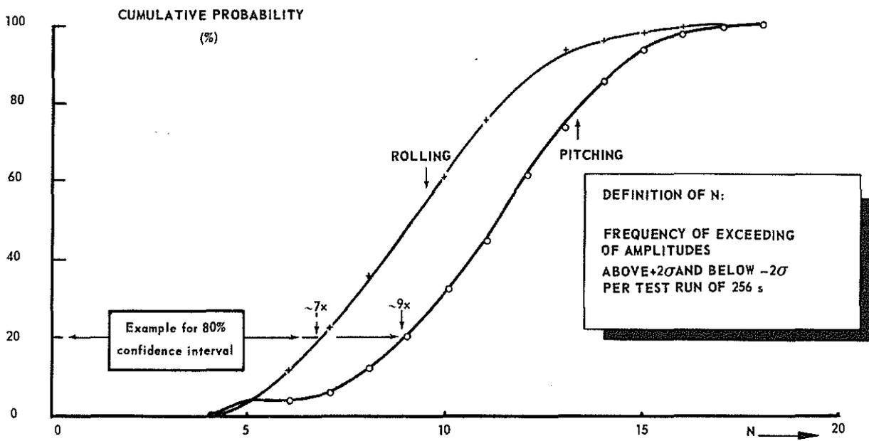
Fig. 12 Cumulative probability distribution of amplitudes exceeding  $+2\sigma$  and  $-2\sigma$  levels, based on 44 test runs
