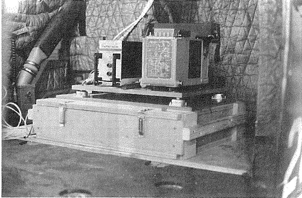
Fig. 5 Arrangement of Hussenot-Beaudouin recorder, engine torque signal conditioner and lead ballast weight container in the helicopter
