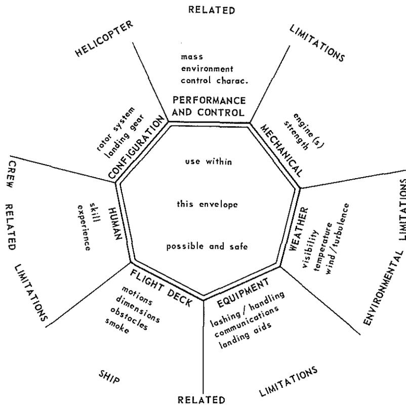
Fig. 1 Various factors limiting the operation of helicopters on board ships
