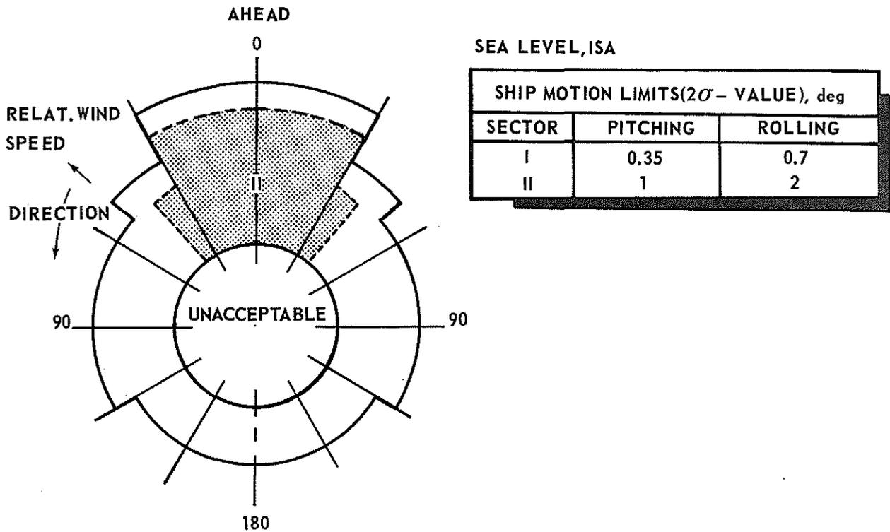
Fig. 11 Take-off and landing limits for day-time, max. helicopter take-off weight
