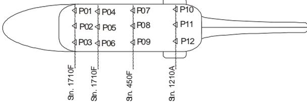
**Fig. 11 Pressure transducers' location**
