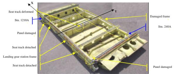
**Fig. 9 Main damages location**
