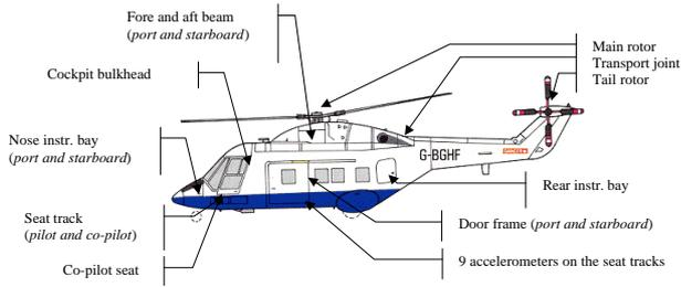
**Fig. 10 Accelerometers' location on the test specimen**
