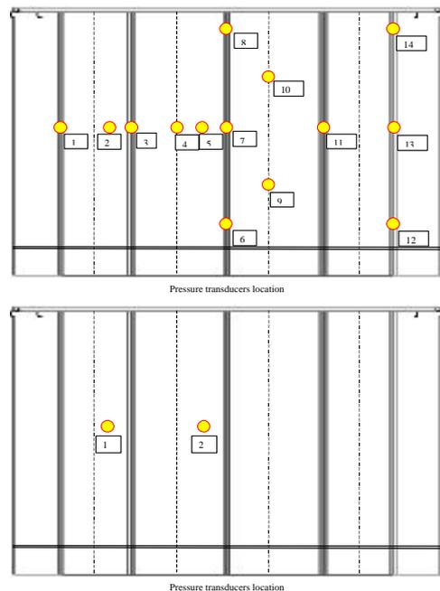
**Fig. 5 Pressure transducers and strain gages location**
