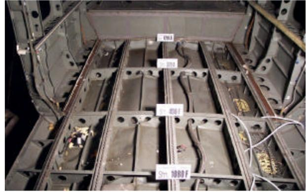
**Fig. 21 Sub-floor inner deformations**
