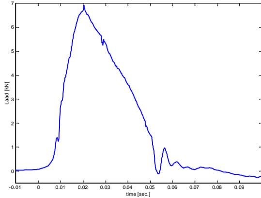
**Fig. 19 Compressive load in ATD spine**
