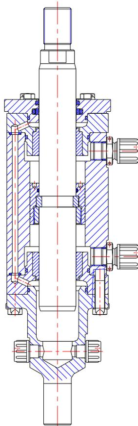
Figure 7. Short-stroke hydraulic actuator 50 KN\*60 mm
