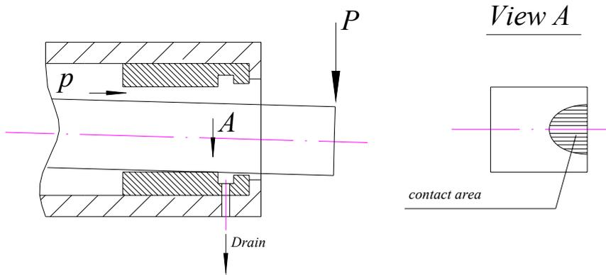
Figure 2. Contact within rod and barrel
