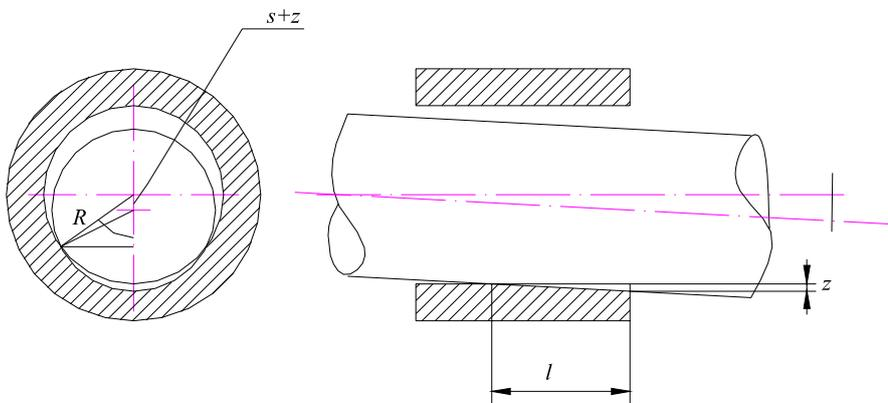
Figure 3. Calculation of rod actuator bearing
