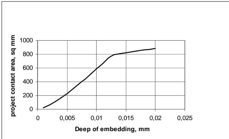
Figure 5. Calculate diagram project contact area relationship on deep of embedding
