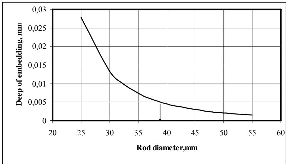
Figure 4. Relation of embedding depth of the bush edge to the rod diameter
