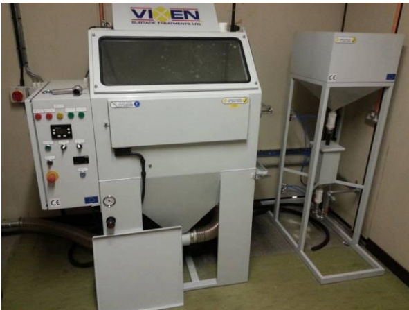
Figure 9: The blade erosion rig developed for this programme in situ in the materials laboratory at AgustaWestland, Yeovil. (image courtesy of AgustaWestland)
