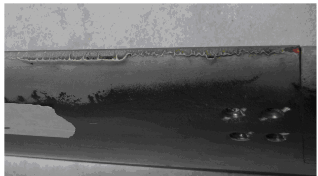
Figure 2: Tail rotor blade showing severe erosion and perforation of the leading edge. (image courtesy of AgustaWestland)
