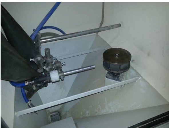
Figure 10: Internal view of Blade Erosion rig showing rotating sample carrier and ejector nozzle. (image courtesy of AgustaWestland)
