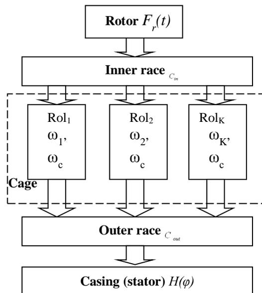
Figure 1. Bearings component interaction chart
