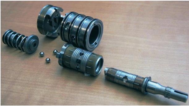
Fig. 5 : Goodrich Rotary Valve Components
