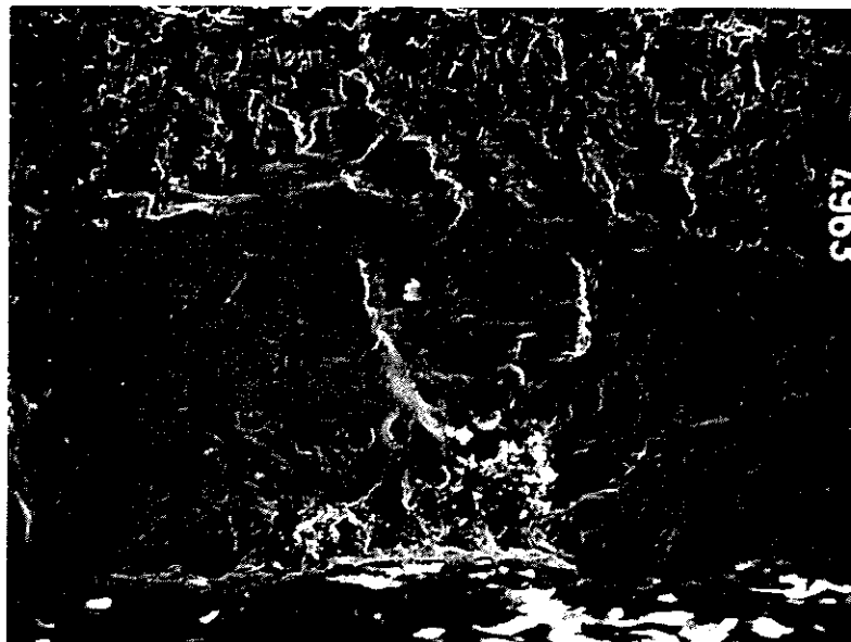
(b) Detail of figure 3a: corrosion pit at fatigue initiation site (x180)
