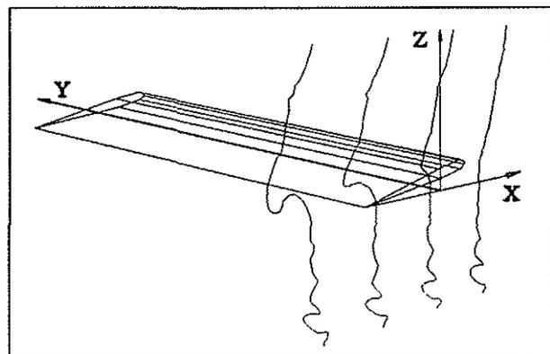
Fig. 6 3D reconstruction of the tip vortex roll-up
