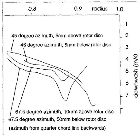
Fig. 15 Initial measurement of downwash velocities (at different azimuthal and vertical positions)
