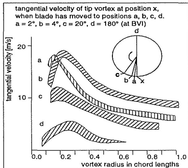
Fig. 11 Measurement of tangential velocities in the developing tip vortex
