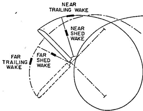
Fig. 1. Wake geometry showing near and far trailed and shed wakes.
