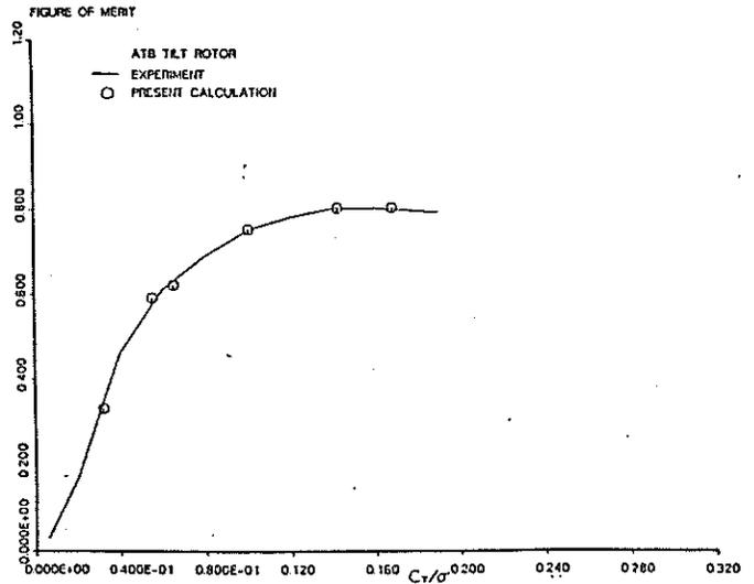
Fig. 6. Comparison of computed figure of merit for tilt rotor on hover compared to experimental data of Ref. 11.
