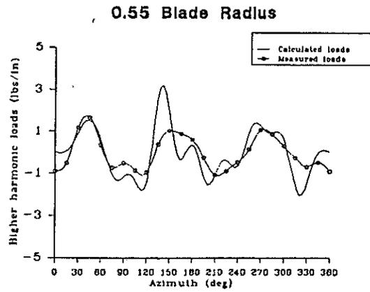
Fig. 4. Computed blade loading as a function of azimuth for same flight condition as Fig. 3, compared with experimental data of Ref. 8. Column 1: total loads, Column 2: harmonic loads above 2nd.
