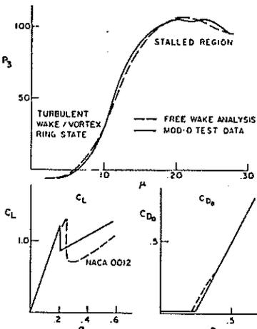
Fig. 8. Comparison between measured performance of Mod-O wind turbine (Ref. 13) and free wake analytical results with lift and drag schedule as shown.  $P_3$  in kW.
