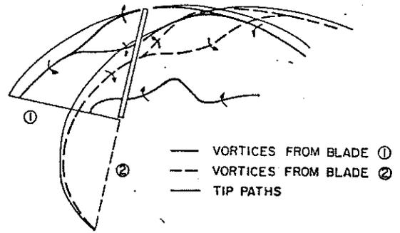
Fig. 2. Sketch of wake geometry at critical intersections using three trailed vortex model.
