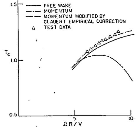
Fig. 10. Wind turbine performance predictions in turbulent wake/vortex ring state and comparison with experimental results of Ref. 14 and with empirical correction of 1976 by Glauert.
