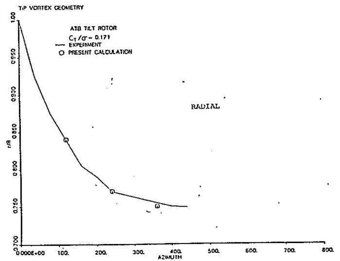
Fig. 7. Experimental and computed wake geometries for rotor of Fig. 6.
