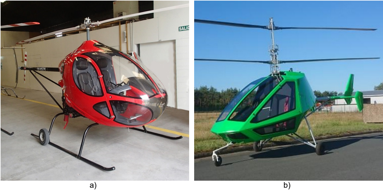
Fig.1. The small weighted helicopters: a – single rotor helicopter Cicare CH-8 (Argentina), MTOM-480kg, b – coaxial helicopter Rotorschmiede VA-250 (Germany), MTOM-500kg
