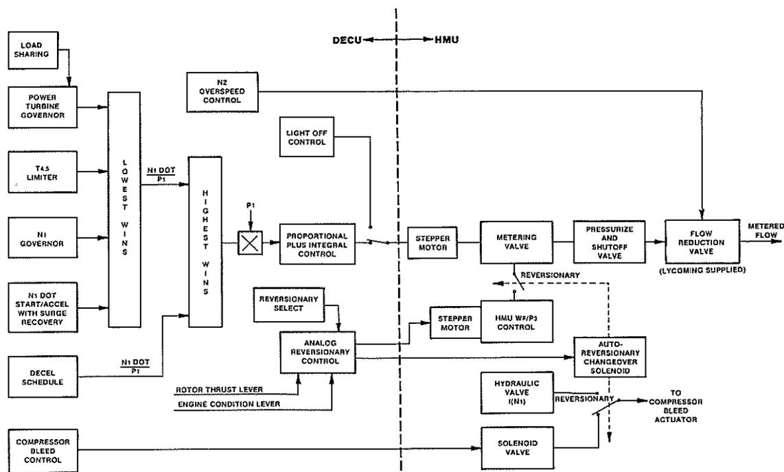
Figure 5 FADEC SIMPLIFIED FUNCTIONAL BLOCK DIGRAM
