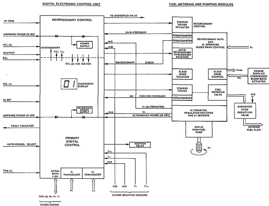
Figure 4 FADEC INTERFACE BLOCK DIAGRAM
