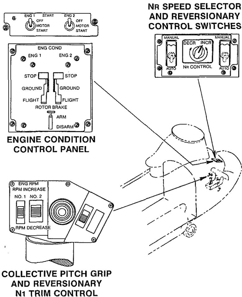
Figure 10 HC Mk1 COCKPIT LAYOUT WITH FADEC
