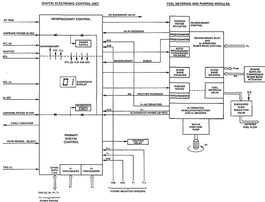
Figure 4 FADEC INTERFACE BLOCK DIAGRAM
