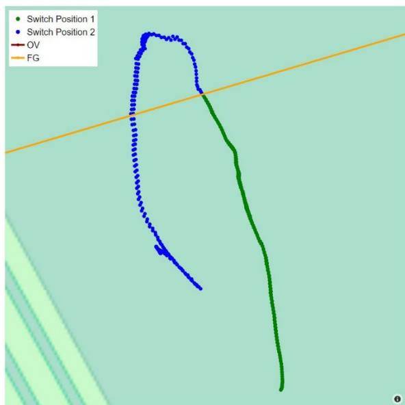
Figure 9 - Zoom on UAV position during geofencing flight test.
