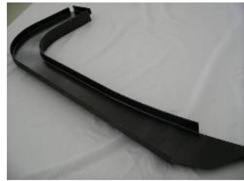
Figure 10: Impregnated curved L-Z-frame
