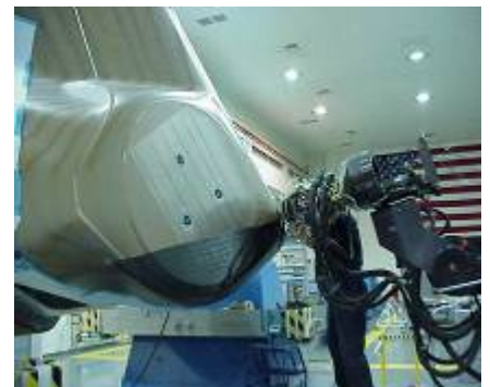
Figure 8: Fibre placement study for fully automated lay-up generation
