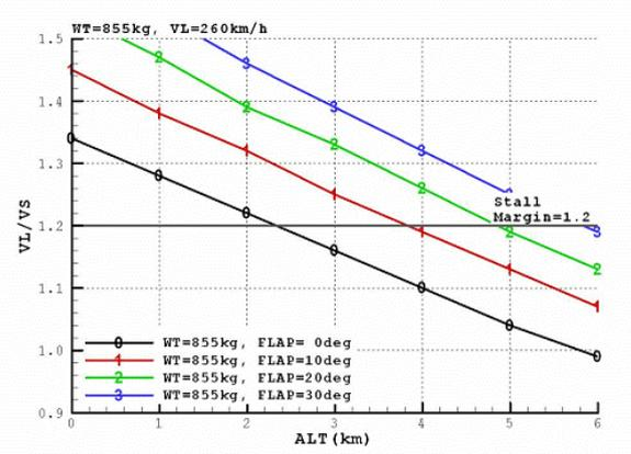
Figure 11: Altitude vs. Stall Margin (Weight=855kg)
