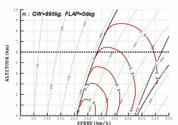
Figure 12: Flight Envelope (Weight=995kg, Flap =0°, Specific Excess Power (PS) & Load Factor (n))
