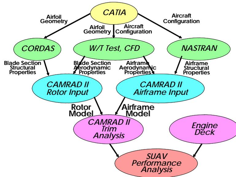
Figure 2: Performance Analysis Process of SUAV Using CAMRAD II
