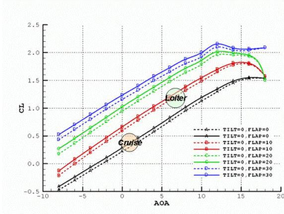
Figure 4: Lift Curve of SUAV
