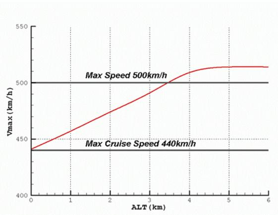
Figure 7: Altitude vs. Max. Speed
