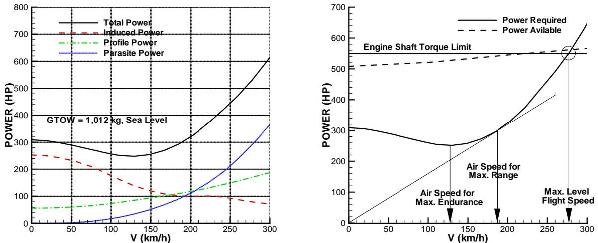
Figure 13: Speed vs. Required Power
