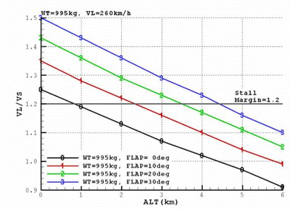
Figure 10: Altitude vs. Stall Margin (Weight=995kg)
