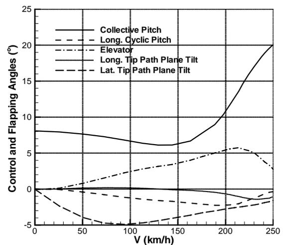
Figure 15: Control and Flapping Angle Variation along Corridor Center (Flap=25°)
