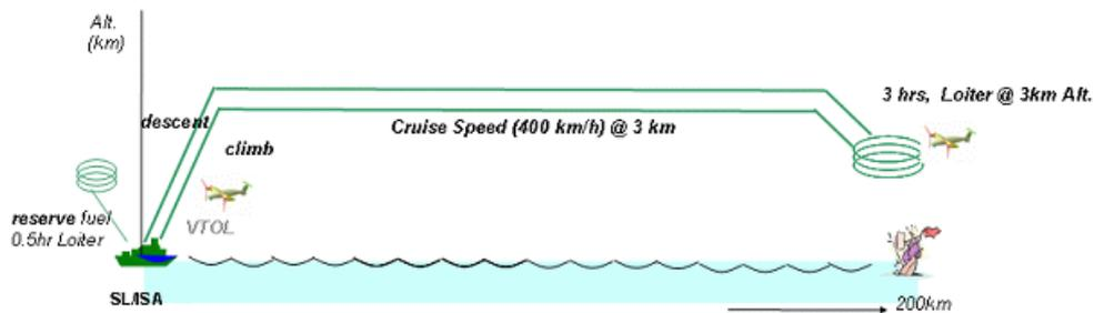
Figure 16: Standard Mission Profile of SUAV (Emergency Catch Up)
