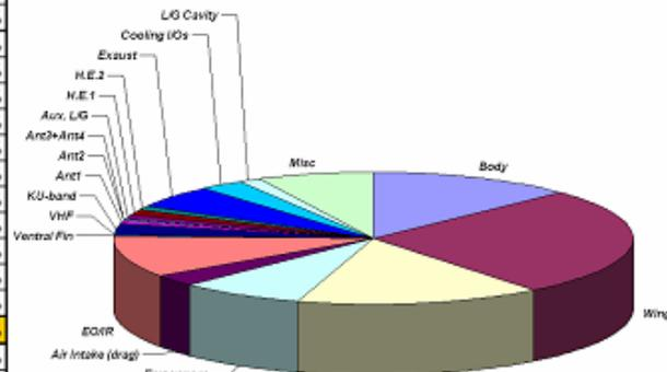
Figure 3: Minimum Drag Coefficient Breakdown
