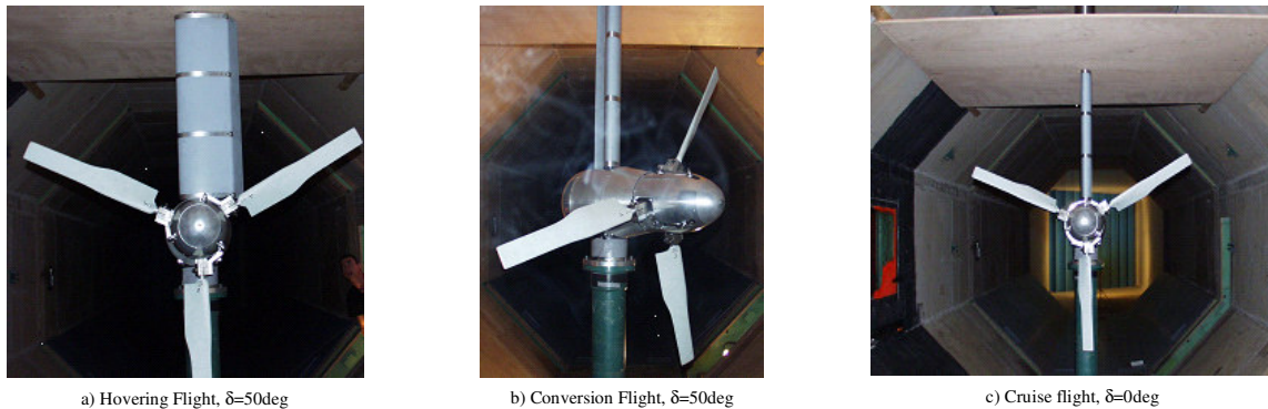
Figure 1: Views of the tilt-rotor set-up in different flight configurations
