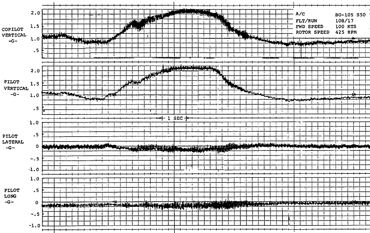
Figure 17. Cockpit vibration During A 60° Banked Turn
