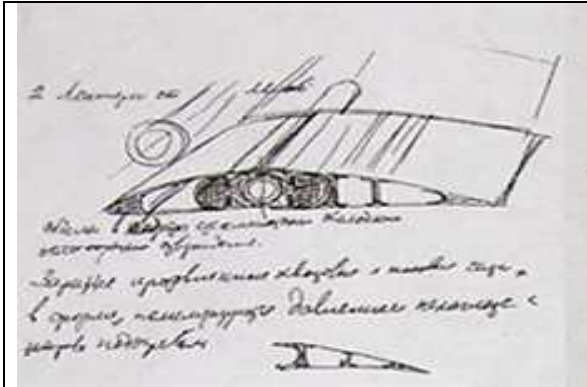
Figure 5: Sketch of composite blade layout. M.L. Mil was the first to offer a steel tubular spar combining all the structural members by filling them with foamed polyurethane and glass fibre reinforced plastic.
