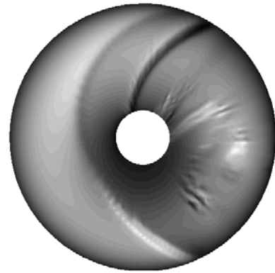
(a) Sectional thrust distribution (present freewake)
