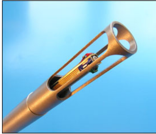
Figure 2. Microflown 3D sound probe. Three particle velocity elements (red, blue and green) are combined with a 1/10" pressure microphone
