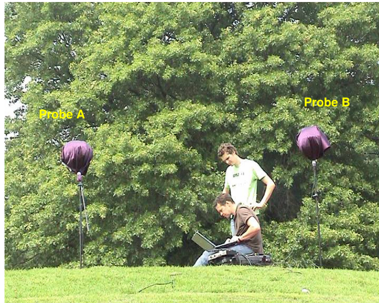
Figure 7. Outdoor measurement using windshield protection
