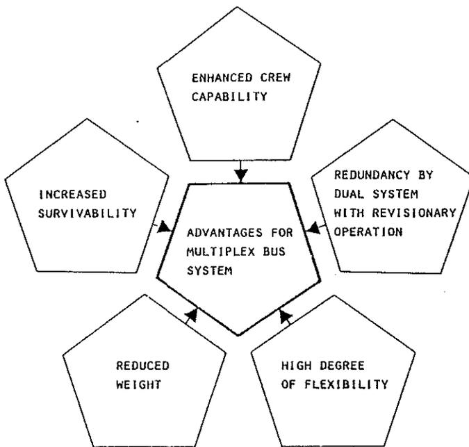
Fig. 18: Characteristics of bus system
