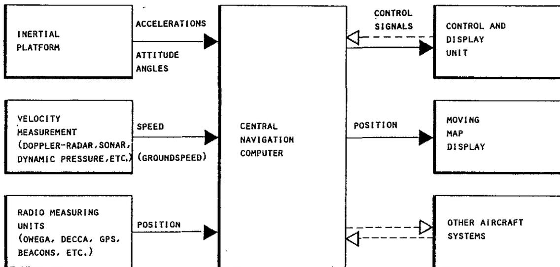
Fig. 7: Integrated navigation system diagram
