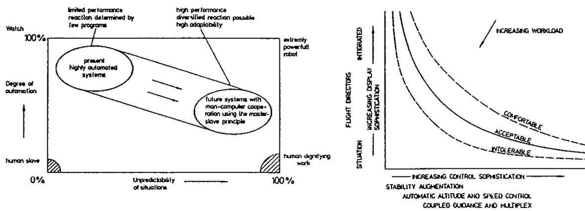
Fig. 5: Interdependence between complexity and automation
