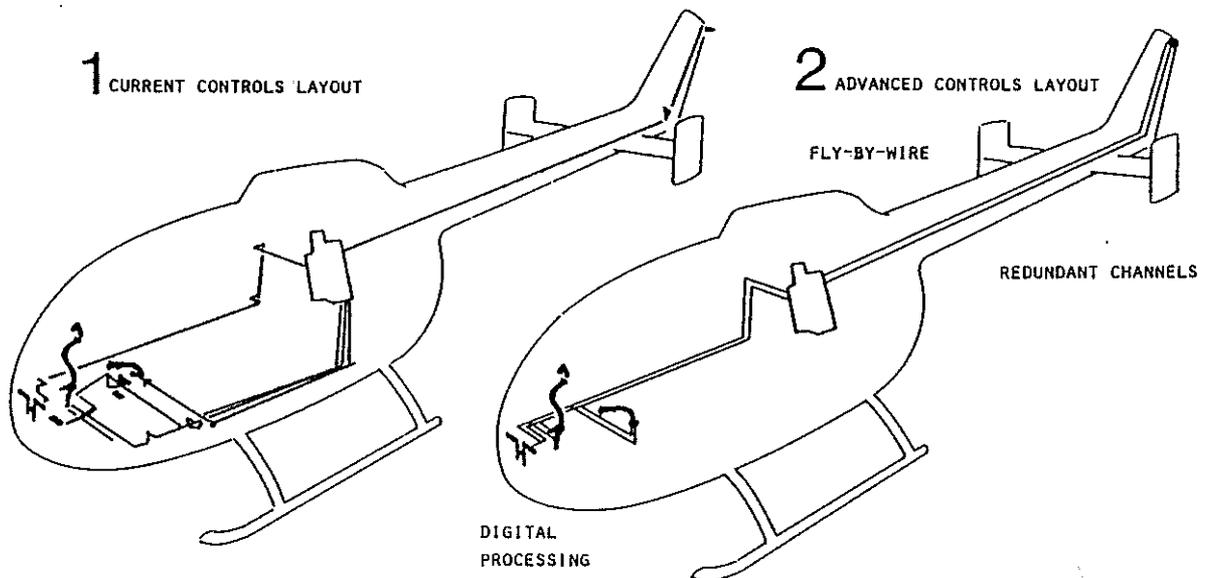
Fig. 15: Comparison mechanical - electronic flight controls
