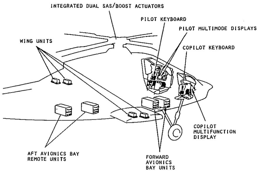
Fig. 23: Remoted terminal units installation
