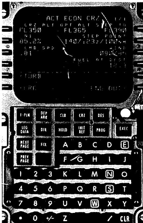
Fig. 19: Control and display unit
