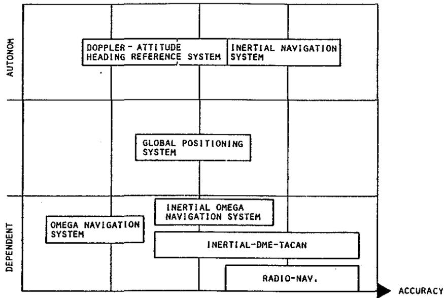
Fig. 6: Characteristic of navigation systems
