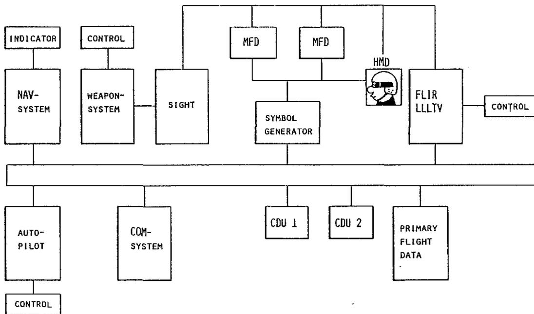
Fig. 17: Multiplex bus system architecture
