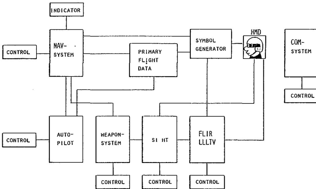
Fig. 16: Conventional system architecture
