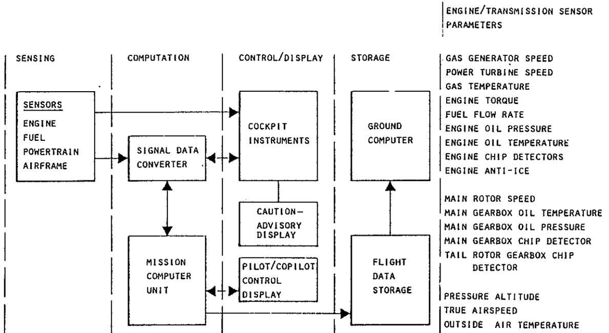
Fig. 14: Monitoring flow diagram
