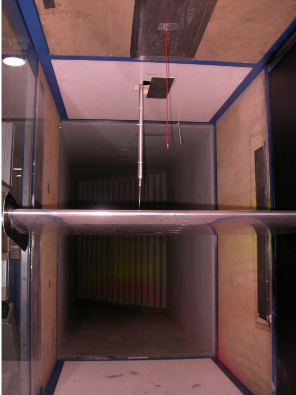
Figure 1: NACA 23012 blade section model inside the wind tunnel test section.
