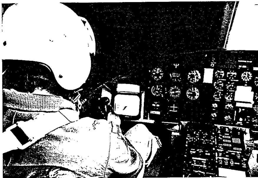
Fig. 2 Experimental head-down display integrated in the left cockpit panel of a Bell UH-1D helicopter.
