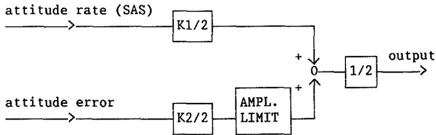
By selecting the amplitude limit threshold to equal half of allowed digital range, the attitude error path will not lose any dynamic quality (with respect to the previous implementation), and thereby the SAS can have complete control of the output signal.
