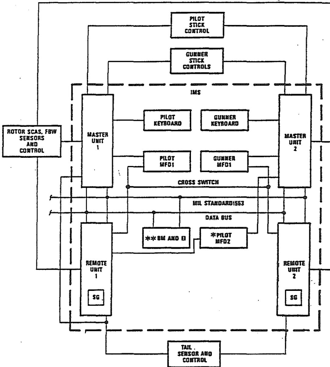
Fig. 3.1 IMS Hardware Flight Control System Configuration
