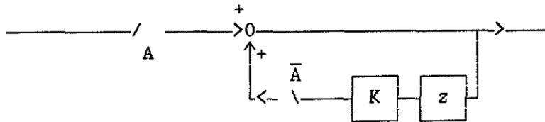
Switch A opens when the function is deactivated, forcing the input to zero ( $\bar{A}$  closes). The gain K is less than 1 and determines, with frequency processing, the time constant for "wash-out".
